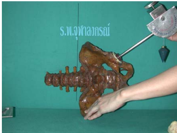
Fig. 2 V-inclinometer with insertion rod attached on the acetabular cup
